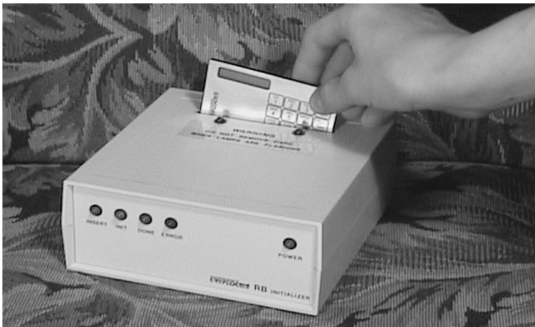
FIGURE 9.9: Token programming device. This programming device or “initializer” accepts an authentication token in the slot on top. Internally, the device contains probes that touch a set of contacts on the card. Each card must be programmed individually. The programming process loads a base secret into the token and configures it for any site-specific features, like preferred password formatting. This is an older programming device built by CryptoCard.
