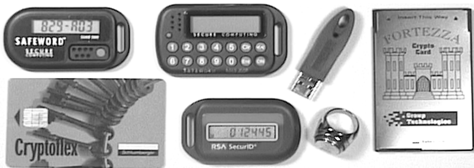
FIGURE 9.1: Seven examples of active tokens. These tokens come in a broad range of shapes, sizes, and technologies. Clockwise from upper left, a SafeWord Silver 2000 one-time password token from Secure Computing; another SafeWord token—the SafeWord Gold 3000; an iKey USB token from Rainbow Technologies; right, a Fortezza crypto card—an NSA-developed PCMCIA card; an iButton ring from Dallas Semiconductor designed to be worn as jewelry; a SecurID one-time password token from RSA Security; a typical credit card-sized smart card produced by Schlumberger.
